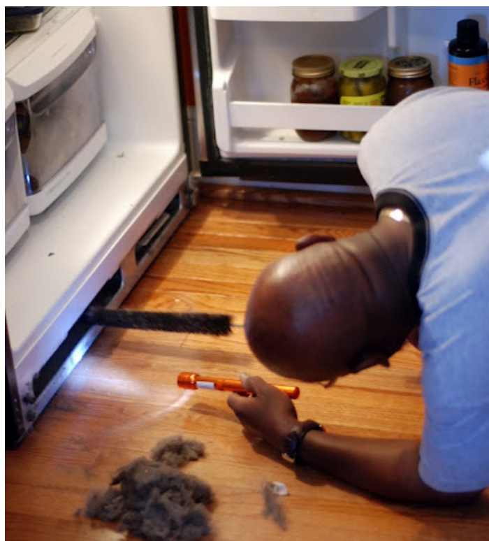
Using a refrigerator brush to clean energy-robbing dust from refrigerator coils.
